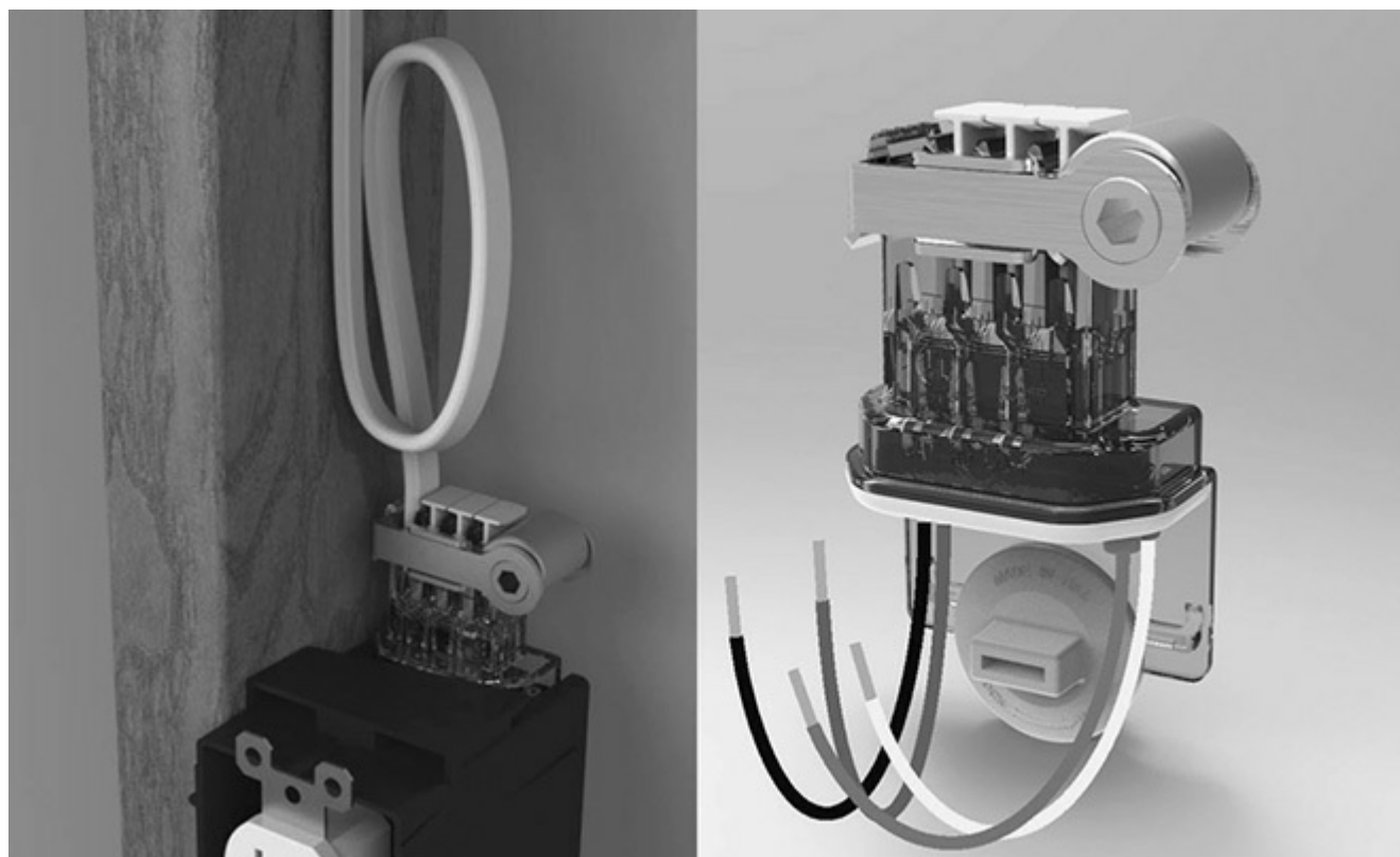
Fig. 314-12. This combination of a termination fitting and nonmetallic box must be part of a listed combination. [Sec. 314.16(B)(2).]
