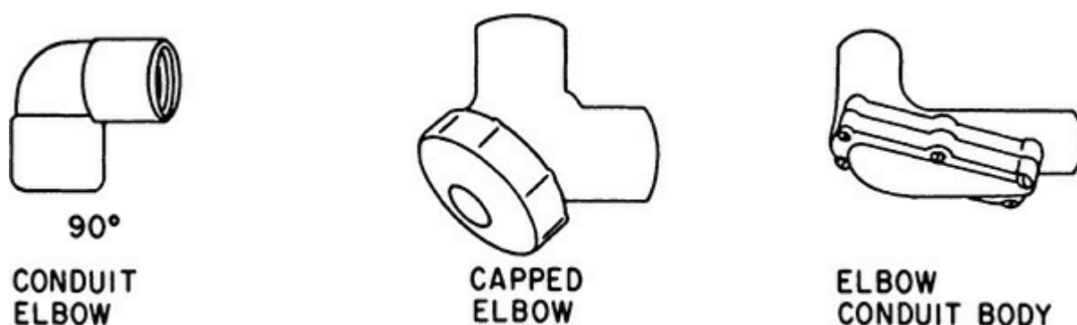
Fig. 501-5. Conduit elbows and similar fittings may be used where wires may be guided into conduit. (Sec. 501.10.) The conduit elbow at the left must only be used where the conductors may be guided through it during installation, and therefore it cannot be used in the middle of a run.
