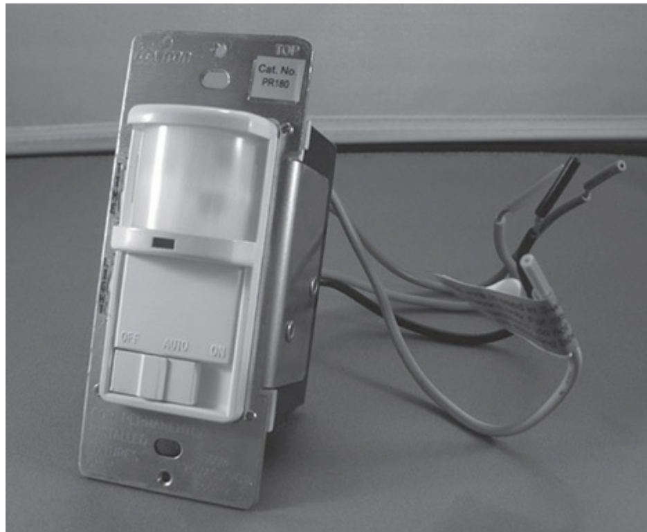
Fig. 404-4. An occupancy-sensor type of switch, designed to replace conventional switches, the four leads are color-coded, and allow for the switch to function as either a single-pole or three-way switch. The fourth lead is green and grounds the switch yoke as well as allowing the electronic controls in the switch to function with the lights off. [Sec. 404.2(C).]
