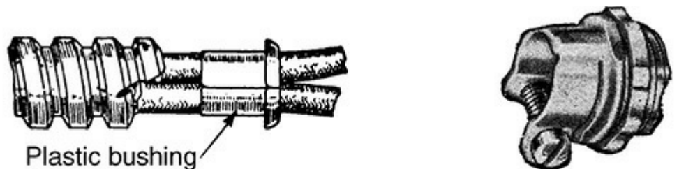
Plastic bushing to protect the conductors in Type AC cable from the sharp edges of the armor.
