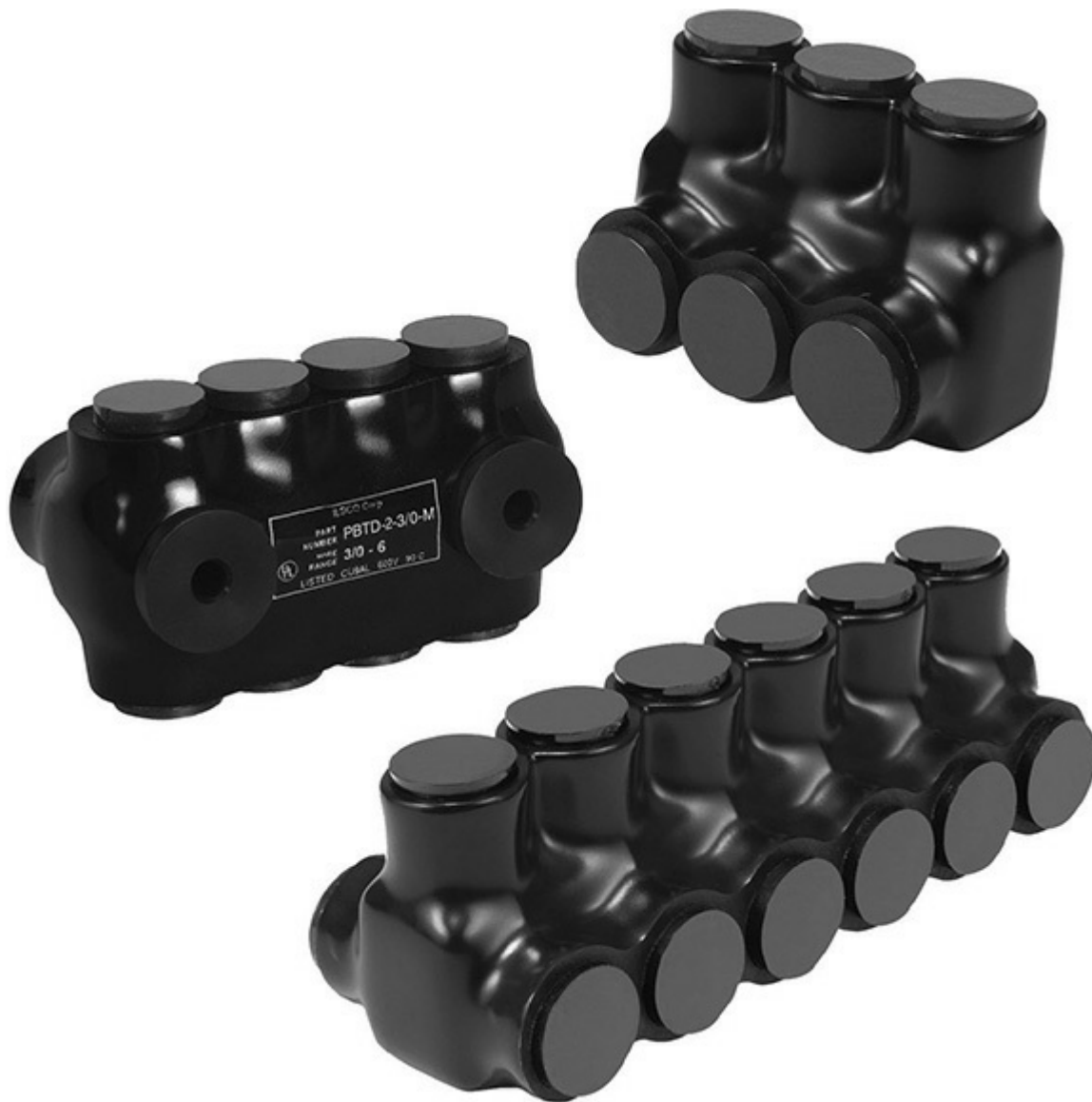
Fig. 110-8. These connectors are listed for a wide variety of finely stranded conductors, including Classes H, I, K, M, and DLO for diesel locomotive use. This vendor has over 50 different configurations with two to six ports and running from 14 AWG up to 350 kcmil, making them suitable for motors up to 200 hp and many other applications. A closely related product line from the same manufacturer covers from 6 AWG up to 750 kcmil. Such terminations routinely involve the use of ferrules to contain the strands, but these do not require them and are therefore reusable without acquiring replacement ferrules. The bearing screw includes a pivoting, nonturning pressure plate that does not cut strands as it tightens. (Courtesy of IlSCO.)
