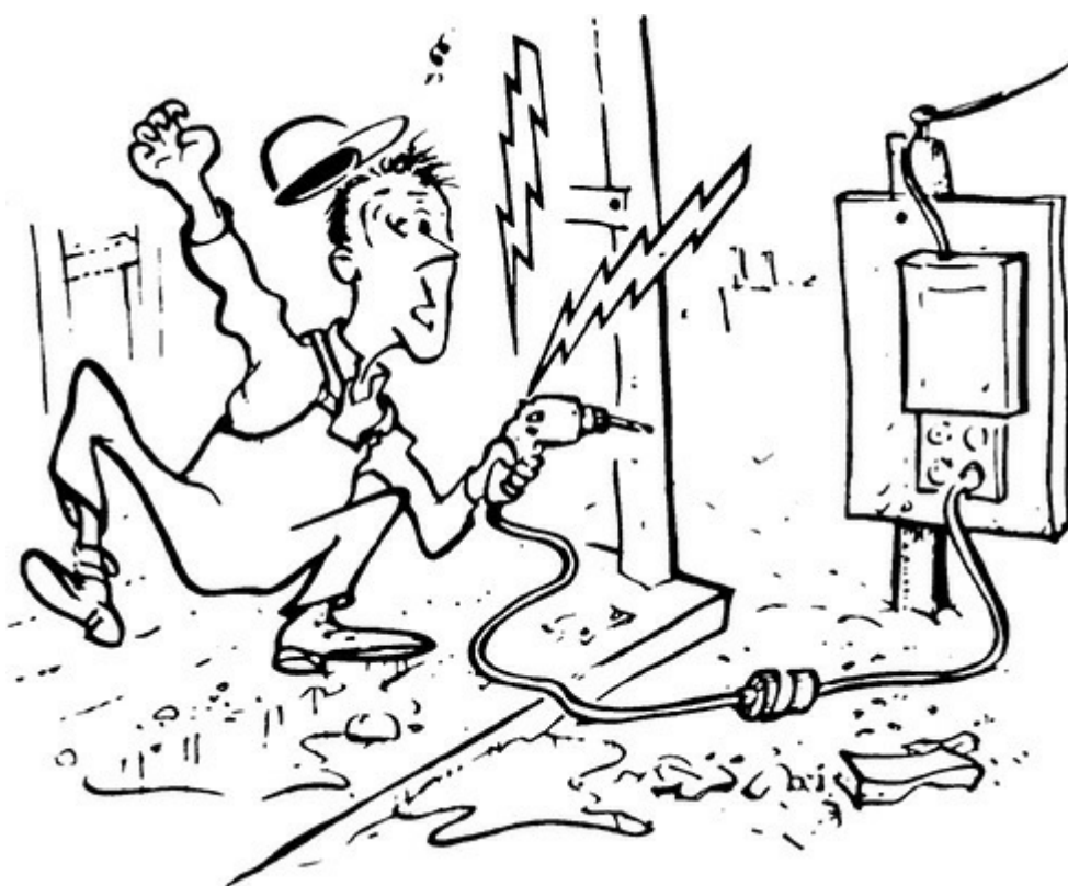
Fig. 100-22. GFCI protection required for temporary power applications, as covered in 590.6, should be listed for temporary power use. Refer to the caption for Fig. 590-13 at the end of Chap. 5 for more information on this topic.
