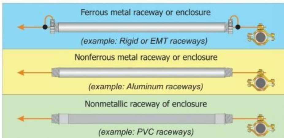
Figure 7.17 Securing and protection from damage and magnetic field
