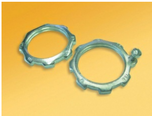
Photo 5.6 Bonding locknut for bonding on the supply side of the service disconnect
