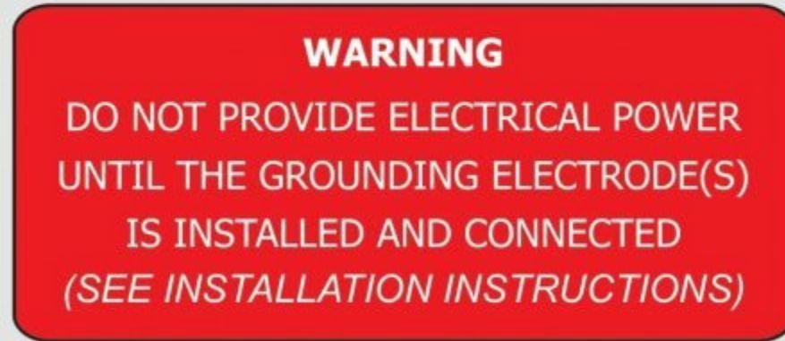
Figure 13.10 Warning label at service equipment of manufactured home
