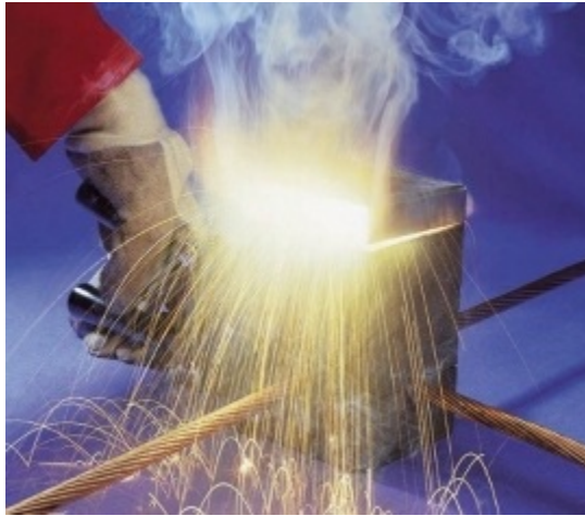
Photo 7.7 Ignition of metallic weld powder
