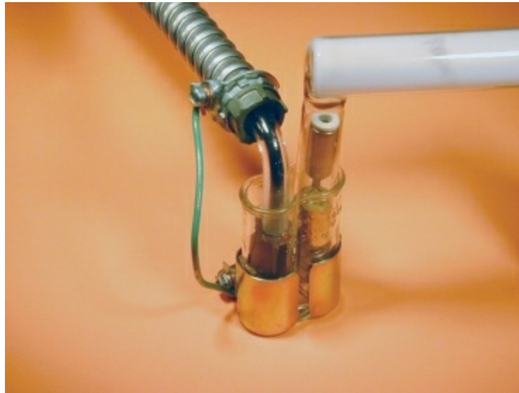
Photo 16.2 Metallic parts shown effectively bonded together
