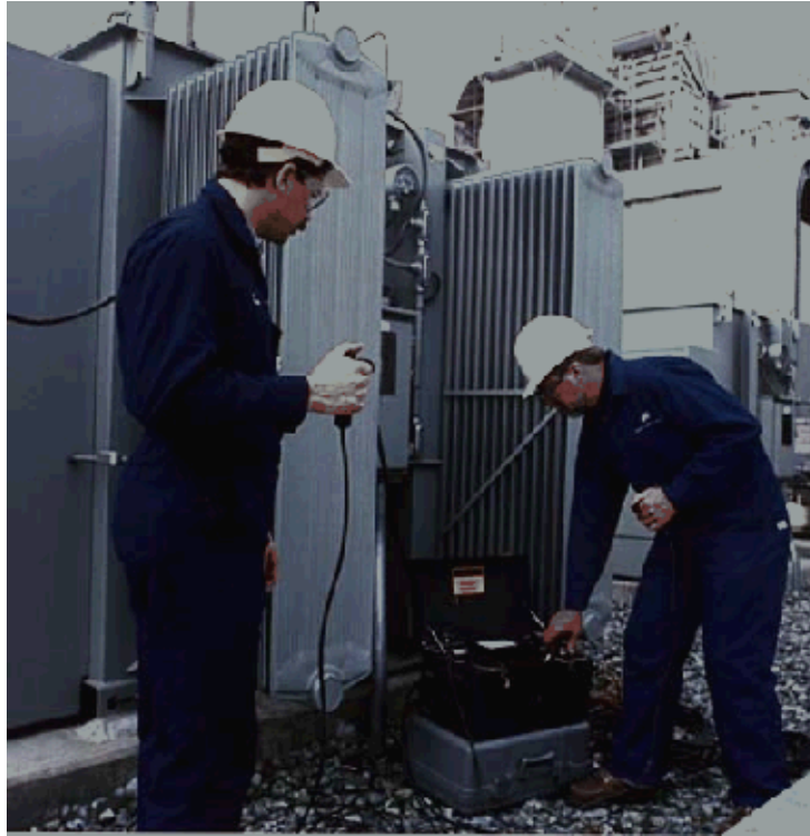
Figure 6-2—Insulation power-factor testing
