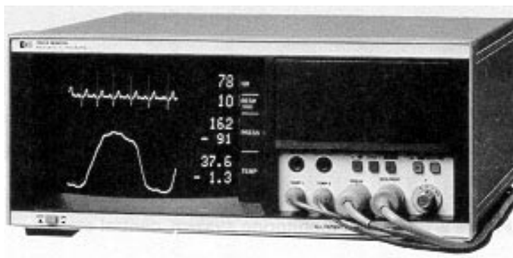
Figure 9-3—Patient monitoring system, bedside station
